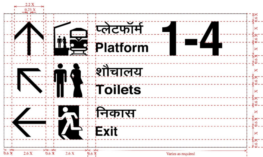
Figure 8: Proportions of Arrow, Pictograms, Text, and Spacing in Signage Boards
