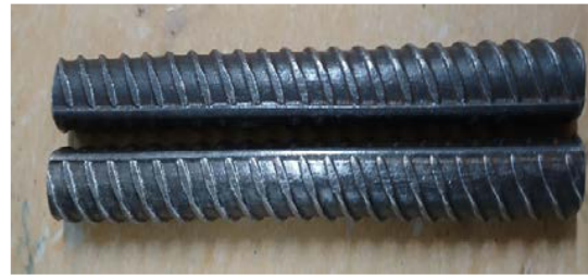
Pictures showing different surface treated TMT Steel reinforced bar
